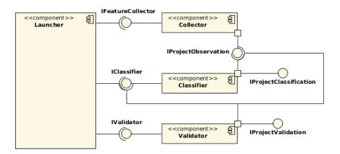
Fig. 1. A component diagram of designed tool. Four main components have been identified: *collector*, *classifier*, *validator*, and *launcher*.
