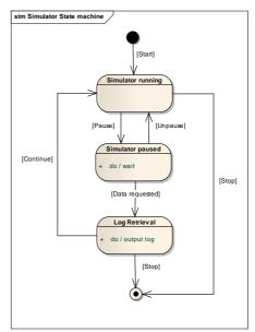
Fig. 4. Example UML State diagram.
