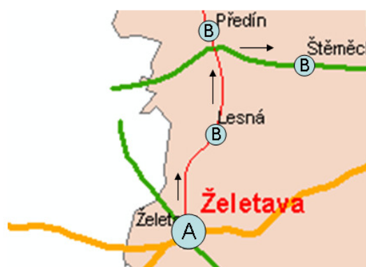
Figure 1: Principle of function Point Distance (A = OUTPUT-FID, B = INPUT_FID)
